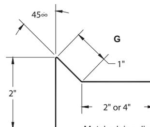
Metal edging dimensions. Use aluminum for edging that contacts secure bar.
