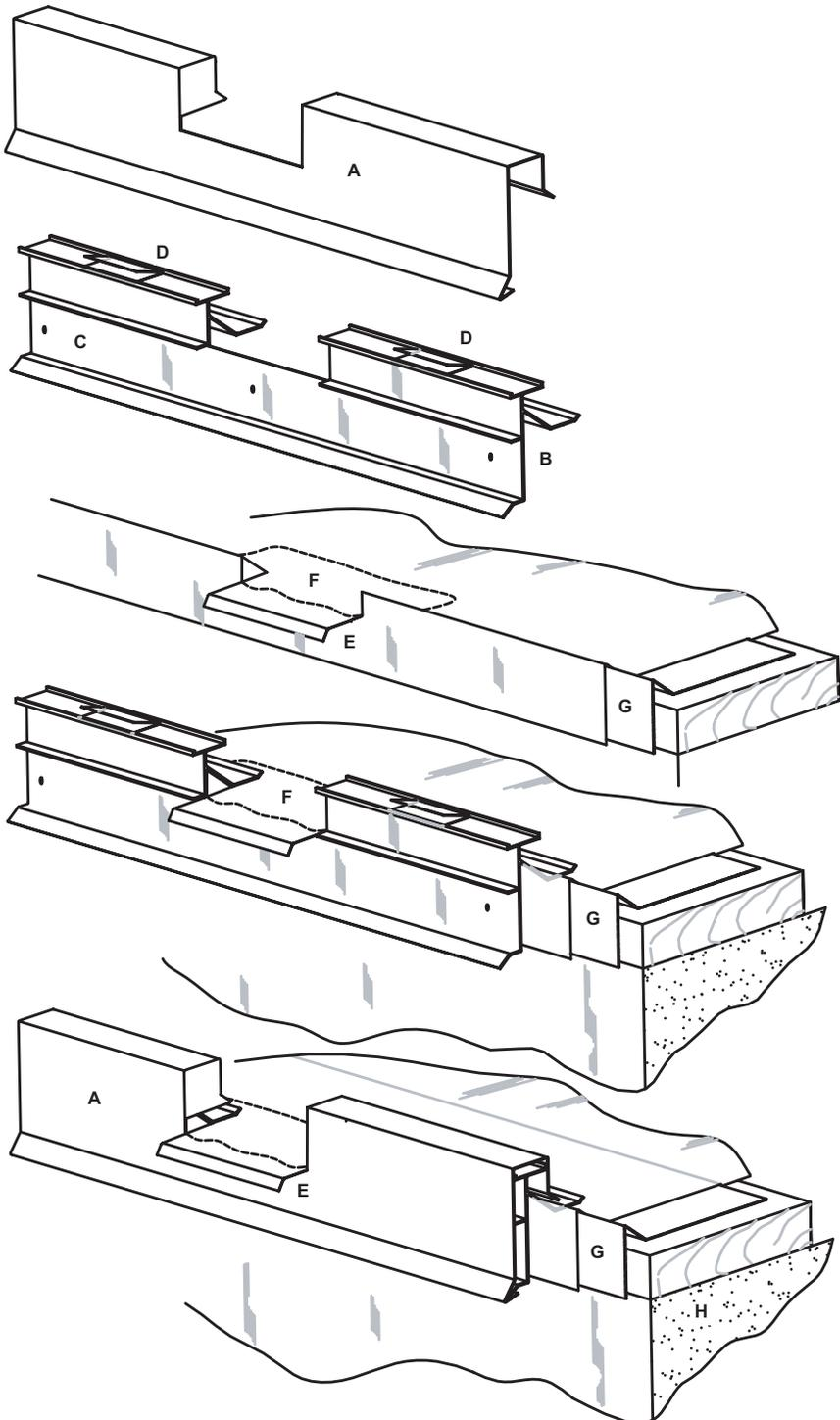
**A** Snap-on decorative aluminum fascia, 30" long, factory notch with welded end caps to cover exposed secure bar and scupper pan. Joint treatment with joining fascias consists of a 3/8" expansion reveal and a 4" wide concealed splice plate.
