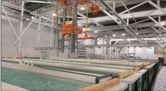
Figure 3. 30 ft anodizing tanks.
