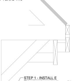
This piece has to be "lanced" before installation. You must use tongs to fold down the top of piece between the slots that has no holes, then put this snug against the plywood and use #10x1" stainless screws to fasten this piece to the plywood. Do not overdrive the screws as this will cause oil canning.
