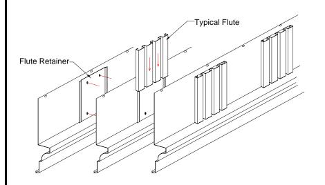
Easy Application; Flutes are installed by simply fastening a flute retainer plate to the frieze fascia. Spacing of flutes is at the designers discretion, however, flutes should be avoided at cornice joints (expansion reveals).
