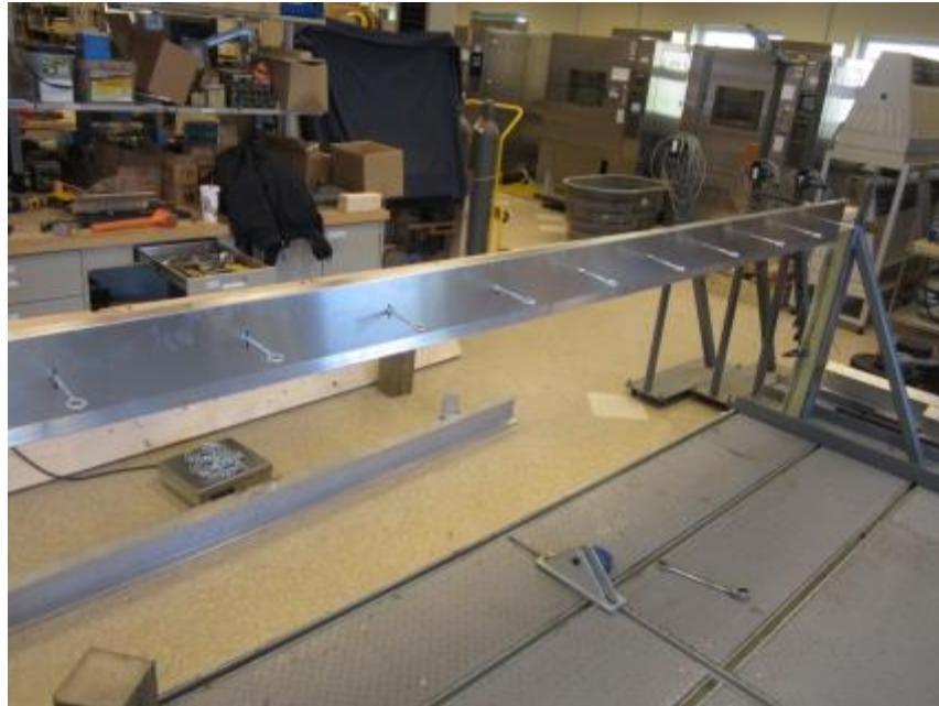
Photo No. 3 ANSI/SPRI Test RE-2, 10 ft Wood Buck, Flashing with Test Eyebolts
