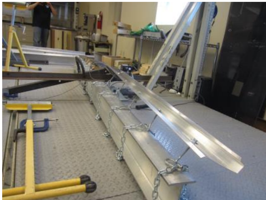
Photo No. 6 ANSI/SPRI Test RE-2, Flashing Pull-Off 6 in Typical Failure Mode: Flashing Pull-Off from Cleat
