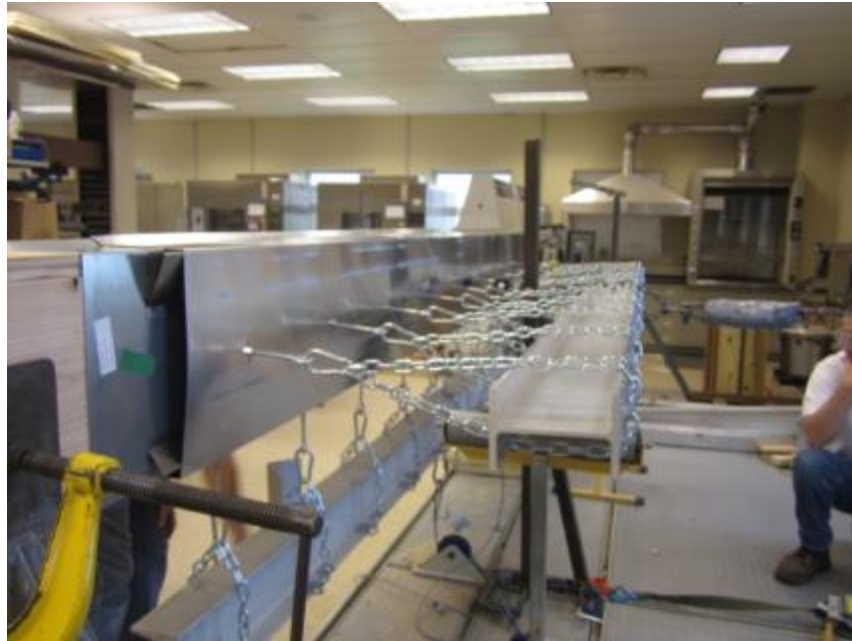
Photo No. 9 ANSI/SPRI Test RE-3, Coping Pull-Off Test In Progress; Tested with Face Down
