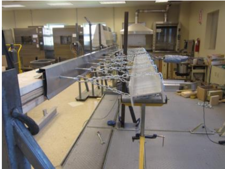
Photo No. 5 ANSI/SPRI Test RE-2, Flashing Pull-Off Test in Progress
