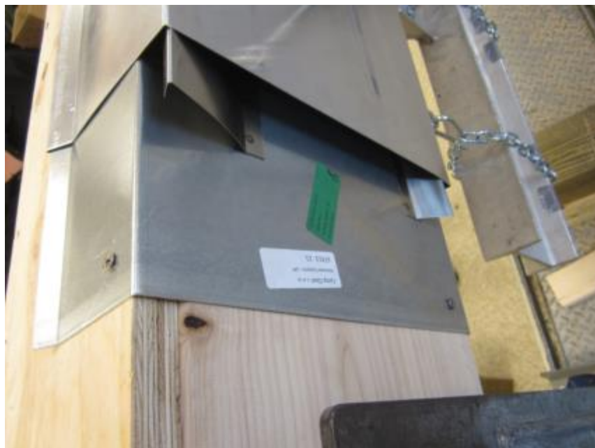
Photo No. 8 ANSI/SPRI Test RE-3, Cleat Orientation in Worst Case Scenario
