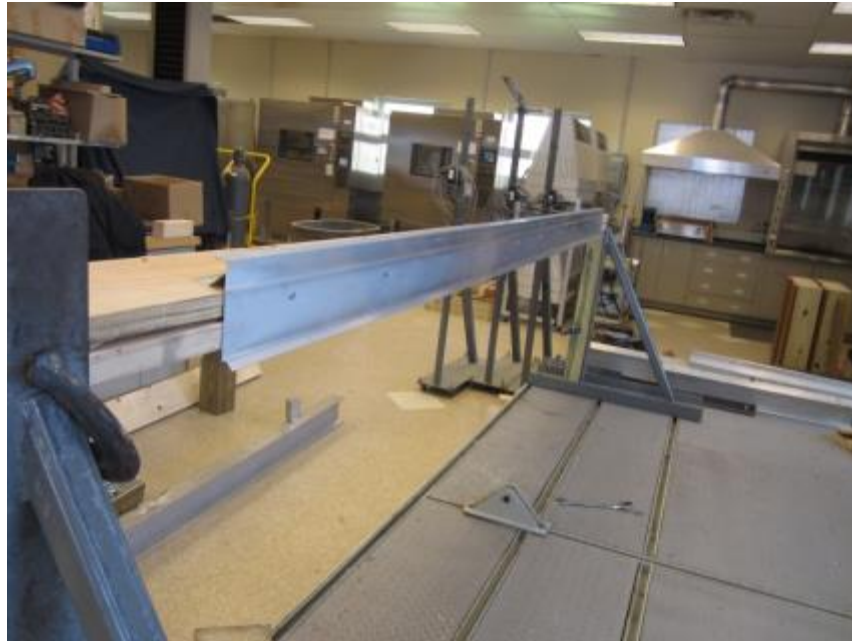
Photo No. 1 6 in Cleat for ANSI/SPRI Test RE-2
