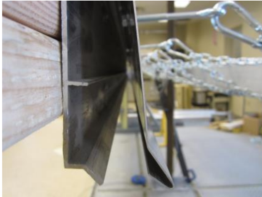
Photo No. 7 ANSI/SPRI Test RE-2, Flashing Pull-Off 8 in Typical Failure Mode: Flashing Pull-Off from Cleat
