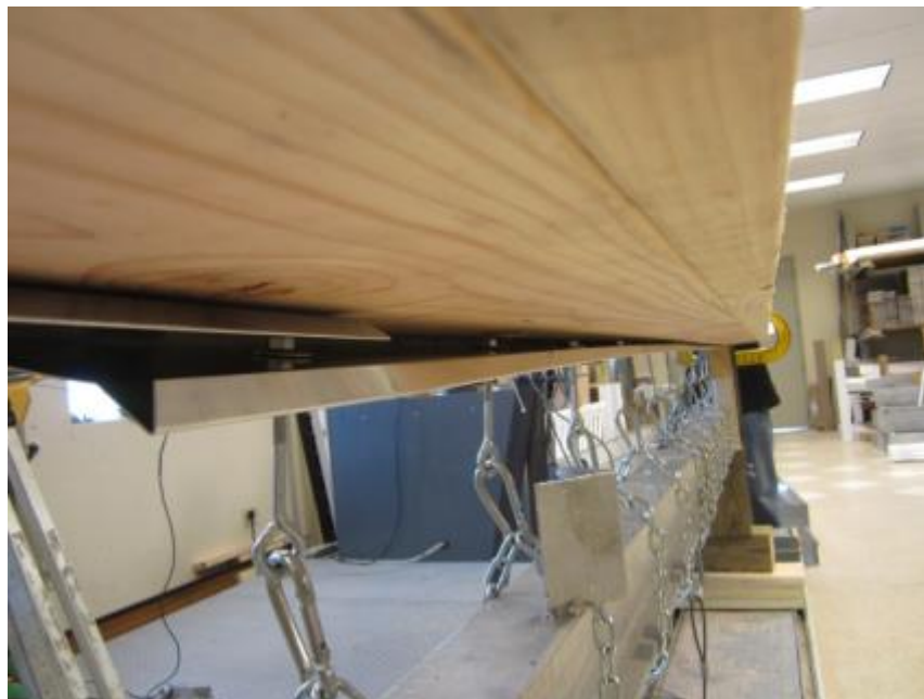
Photo No. 10 ANSI/SPRI Test RE-3, Coping Pull-off Test Typical Failure Mode: Coping Face Lip Pull-Off from Cleat
