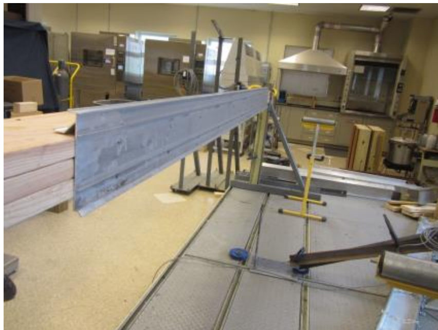
Photo No. 2 8 in Cleat for ANSI/SPRI Test RE-2
